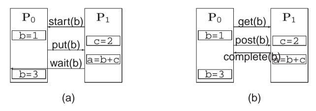
The name *one-sided message passing* is often applied to RMA but this is a misleading term. Instead of paired send/receive calls, we now have transmission events on one side (put, get) paired with *exposure* events (start,wait) and (post,complete), respectively, in MPI-2 terminology, on the other side. It is thus still "two-sided". A variable exposed for a remote get may not be written to by the PE that owns it; and a variable exposed for a remote put may not be read.
