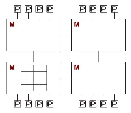
Array is local to one mNode: other mNodes requires remote loads and stores. OK on platforms that are well-balanced in bandwidth and latency for local and remote accesses. **ccNUMA** ensures cache coherence across the aNode.
