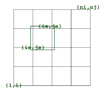
The **computational domain** is the set of gridpoints that are computed on a domain. The **data domain** is the set of gridpoints needs to be available on-processor to carry out the computation, and includes a **halo** of a certain width.
