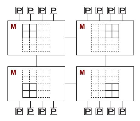
Better memory locality: allocate each block of 4 domains on a separate page, and assign pages to different mNodes, based on processor-memory affinity.
