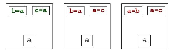
Race conditions occur when one of two concurrent execution streams attempts to write to a memory location when another one is accessing it with either a read or a write: it is not an error for two PEs to read the same memory location simultaneously. The second and third case result in a race condition and unpredictable results. The third case may be OK for certain reduction or search operations, defined within a **critical region**.
